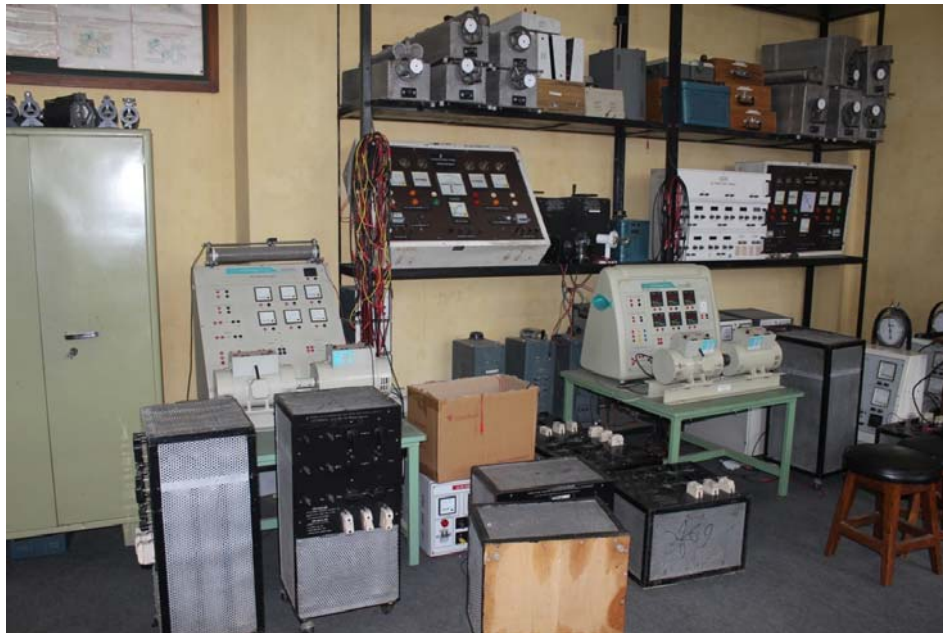
Figure 2.2: Electrical Lab-1 room Specifications-DC Shunt Machines Set and Three phase loads
