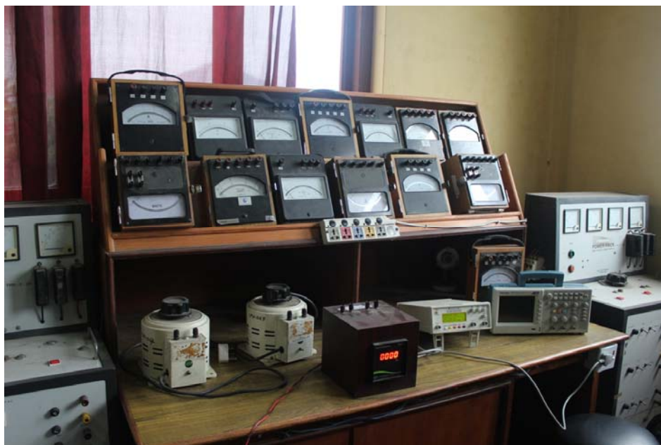
Figure 2.4: Electrical Lab-1 room Specifications-Sources, Indicating Instruments and Small Transformer sets and Function Generator
