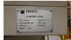
Figure 3. Specification Control Desk
