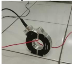
Figure 9. HFCT sensor Specification:
