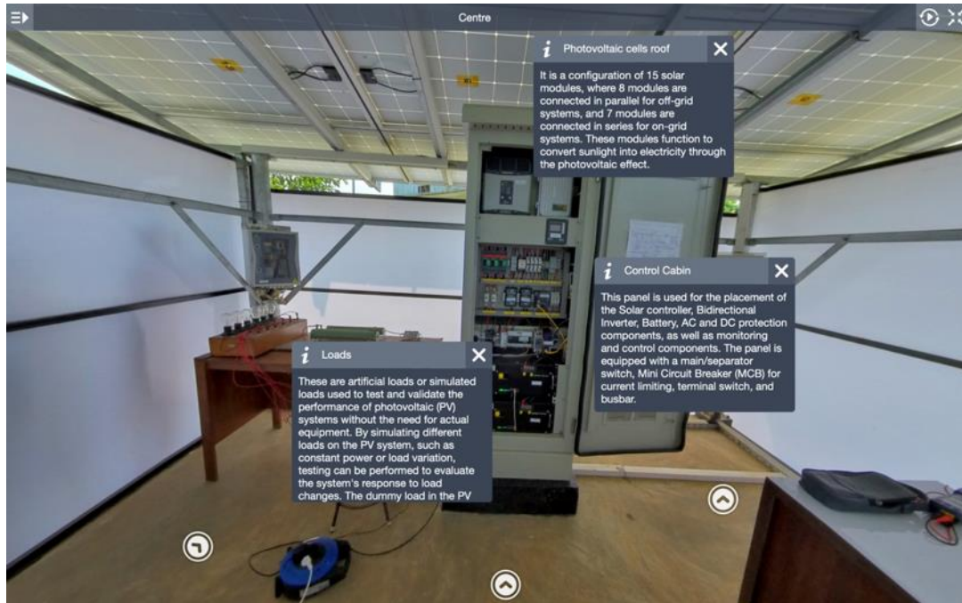
Figure 8 Pop-up on screen description of component and function in the ATM eACCESS laboratory. Main panel board.
